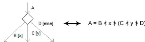
**Fig. 6.** Example Mapping of a Decision Node.
